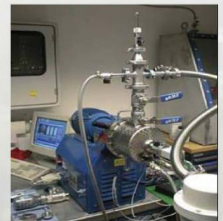
Simoloyer CM01-2lm, 2 liter vessel, air-lock, water-cooling, cycle operation 900/1300 rpm ...
