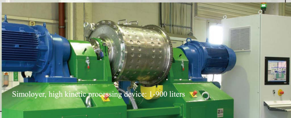
Simoloyer CM01-2lm, 2 liter vessel, air-lock, water-cooling, cycle operation 900/1300 rpm ...
